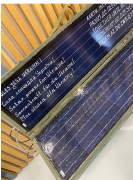
Portable solar panels used to charge communication devices in the Ukraine, back for repair after being damaged by shrapnel incurred in the conflict.
