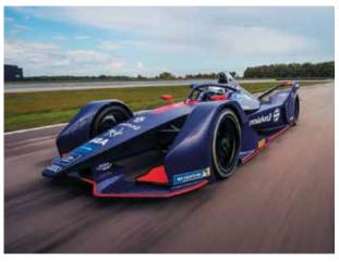
Electric Formula-E racing cars have 250kW of power and will accelerate from 0-100 km/h in 2.8-seconds with a top speed of 280km/h.
